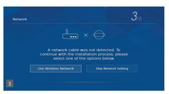
**3. Network setup** You can connect the TV to your broadband router or wireless network in order to take advantage of the Smart functions. If you connect the TV to your router using an Ethernet cable (recommended) this step will be skipped. Follow the on screen prompts to connect to your wireless network. You can set up the Network connection later in the network menu.
